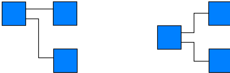
(a) Unbalanced node placement with two edge bends. (b) Balanced node placement with four edge bends.
