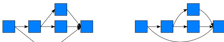
(a) A graph with polyline edge routing. (b) The same graph with spline edge routing.
